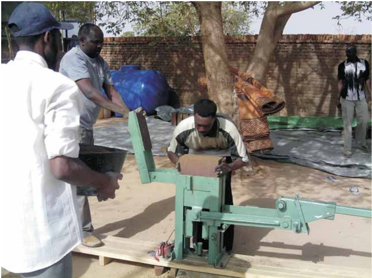
Figure 10. A Stabilized Soil Block (SSB) press of the type being promoted by UN-HABITAT in Darfur
