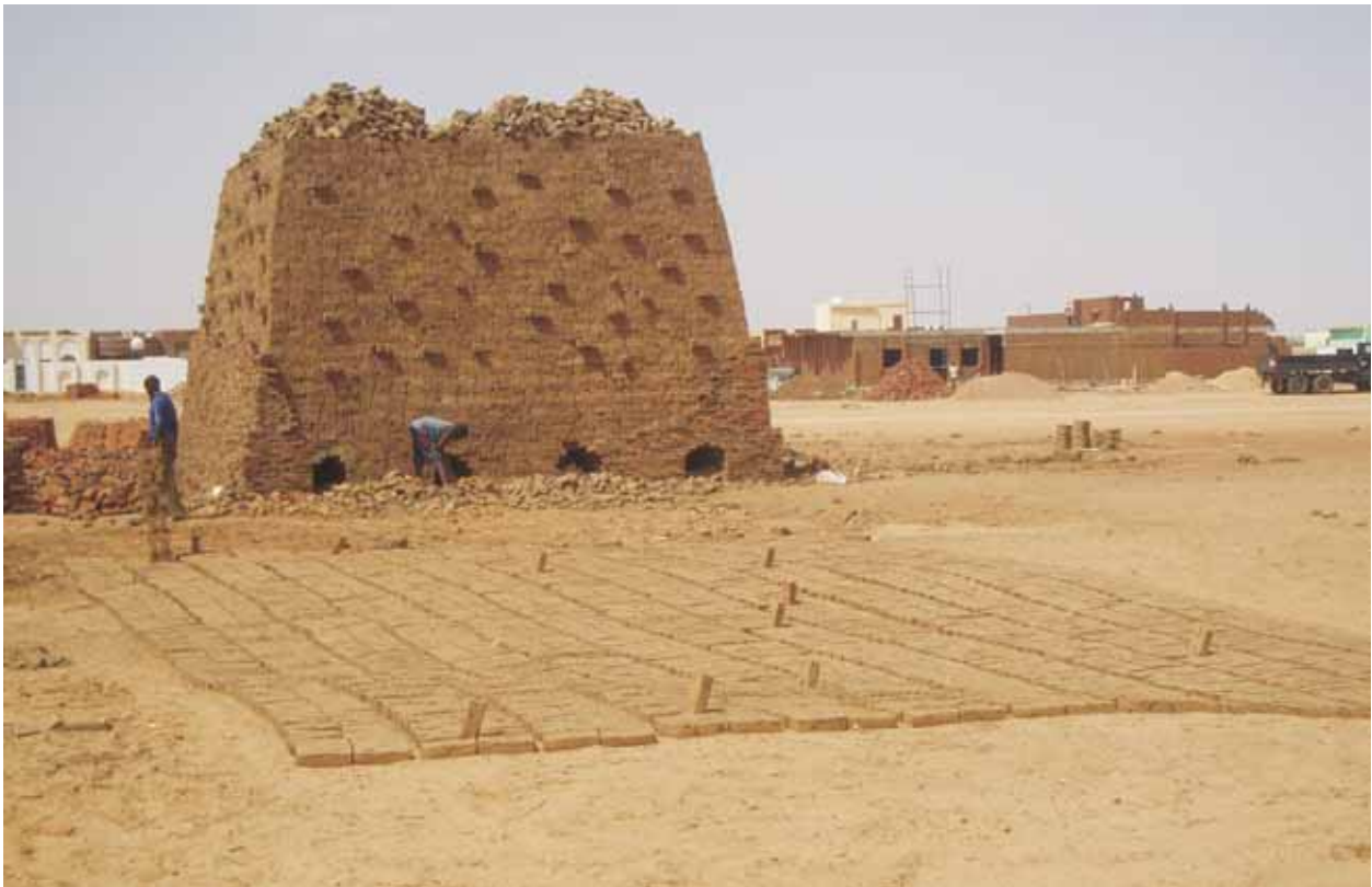
Figure 4. A brick kiln for the new villas being built in El Fasher
